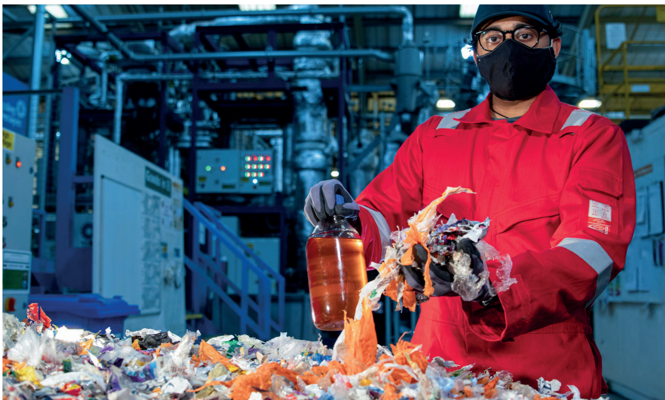
A plant controller at Recycling Technologies, Swindon, UK, holding a bottle of Plaxx® - a liquid hydrocarbon feedstock produced by chemical recycling of waste plastic. After refinement, Plaxx can be used to make virgin quality plastic resin. (Image courtesy Recycling Technologies.)
