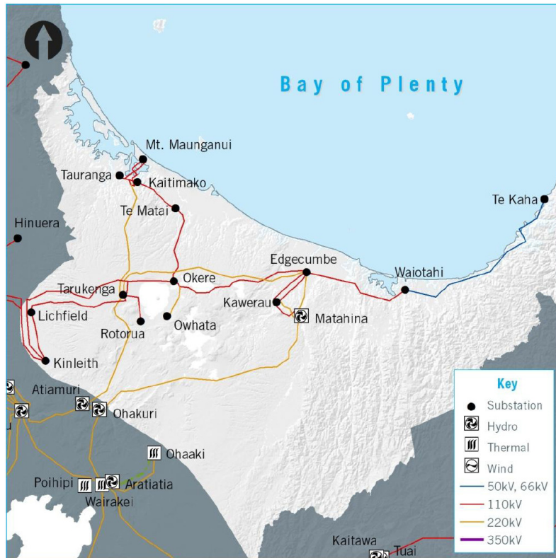
Figure 4: Bay of Plenty electrical grid network [3]
